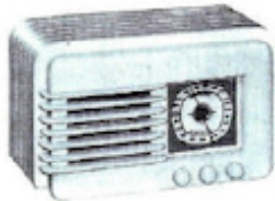
Model 6295P (Code—KING) 6 Tube, latest Superheterodyne Circuit. Dual Band tunes American Broadcasts, Police, Amateurs, Aviation, and Short Wave. Powerful Electro-Dynamic Speaker; High Impedance Litz Coils; Automatic Volume Control; Large Scan Illuminated Airplane Dial. Cabinet in Plaskon Ebony. Dimensions 11 1/2 x 8 1/2 x 7". List Price.....$29.95
